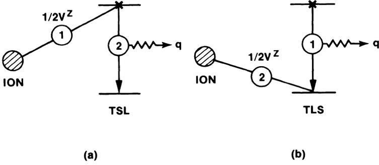
Fig. 2. Two-step processes for diagonal modulation. Directed wiggly lines and circled numbers indicate phonon-emission and the sequence in the perturbation chain, respectively.
