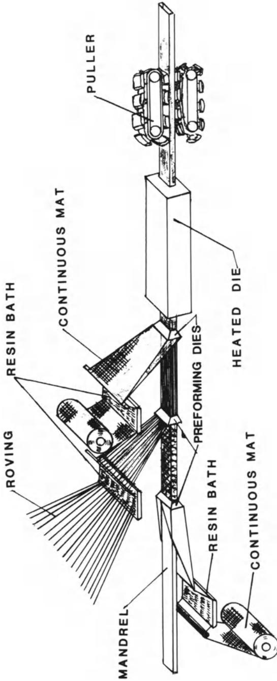
**Figure 1.3** Typical Hollow Pultrusion Process
