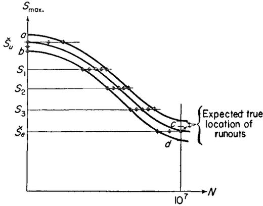
Fig. 20.1.  $P$ - $S$ - $N$  diagram including statically fractured specimens and run-outs.
